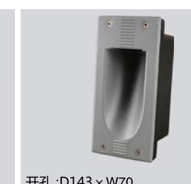
开孔 :D143 × W70 GMD-111A Lamp:LED 1 × 3W Size:D70 × W145 × H65
